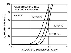
Figure 5. Transfer Characteristics
