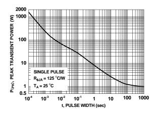
Figure 12. Single Pulse Maximum Power Dissipation
