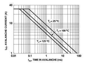
Figure 9. Unclamped Inductive Switching Capability
