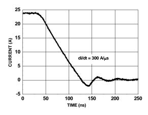
Figure 14. FDMS0308AS SyncFET body diode reverse recovery characteristic
