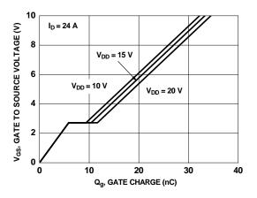
Figure 7. Gate Charge Characteristics
