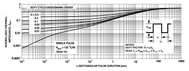
Figure 13. Junction-to-Ambient Transient Thermal Response Curve
