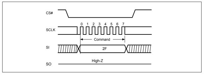
Figure 29. Write Security Register (WRSCUR) Sequence (Command 2F) (SPI mode)
